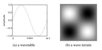
Figure 1: An example of a 1D (a) and 2D (b) lookup table for sound synthesis.
