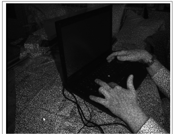
Figure 6: Infrared light patterns projected by the Kinect. (c) CC-BY-SA-3.0, via Wikimedia Commons.
